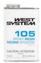
excellent moisture resistance. West System 105 Resin is formulated without volatile solvents and does not shrink after curing. It has a relatively high flash point and no strong solvent odour, making it safer to work with than polyester or vinyl ester resins. Resin viscosity is approximately 1000 centipoise (cp) at 72 F (22C),
