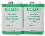
together, will expand to approximately 25 times its volume at 21° C. It has a density of 2 lb. per cubic foot and is used to fill cavities and voids, insulation for tanks and holds, and as floatation for docks, etc. Size: 8L
