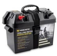
box. Built-in battery meter displays current "state of charge". Includes two 12-volt accessory plugs, and 2 manual reset circuit breakers (10 amp for accessory plugs and 60 amp for trolling motor). Fits group 24- and 27-size batteries.
